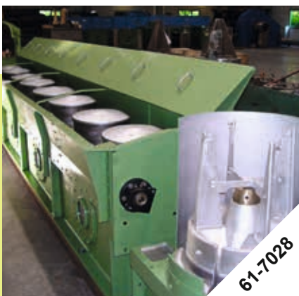
MRB 9-Die rod drawing machine for aluminium wires, MR 9
