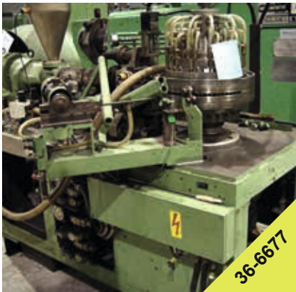
REIFENHÄUSER Coaxial cable inner conductor extruder, SO25,1-20
