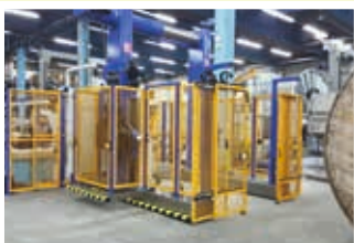
Pay-offs and take-ups: • portal traversing design • bridge type design • column-type design • cantilever-type design
