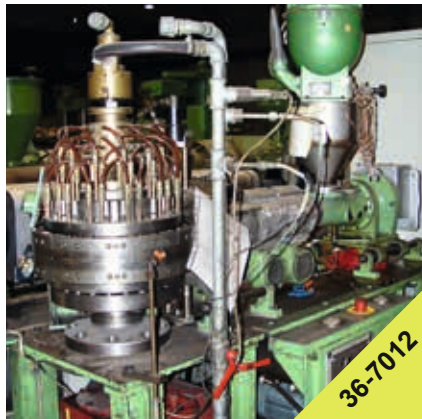
REIFENHÄUSER Extruder for application of spacer discs
