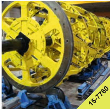
QUEINS 84-Bobbin armouring planetary strander
